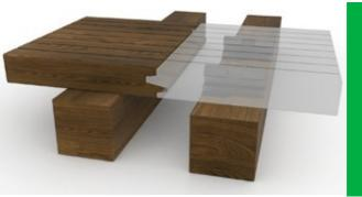
In contrast to traditional construction techniques, with Tantimber Thermowood it is not required to have the ends of the boards fall directly above the joists whether or not end-matching products are used.
