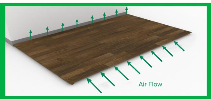
It is important to maintain proper gaps and spacing between all deck components to ensure proper airflow and water drainage in order to allow the wood to breath and not
