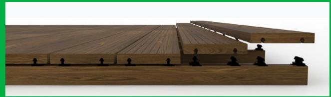
When installed in public areas and for other urban projects, decking may be attached with stainless steel screws, although Tantak Clips are the preferred method. In these applications, the decking should be a minimum of 1" thick.
